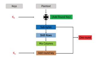
Figure 1. Block structure
