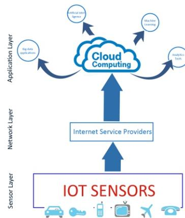
*Figure 1 Architecture of a Cloud based IoT Environment*
